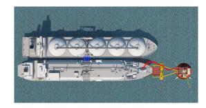
**Cross-dock FSRUs** – segregated berths for LNG ships and FSRUs provide flexibility and improved availability. Spacious 'sea island' concepts can be created to enable a flexible, offshore operation: this allows for adding more vaporizer capacity and further berths for a Floating Storage Unit (FSU) or another FSRU. *Examples: Guanabara Bay Brazil*
